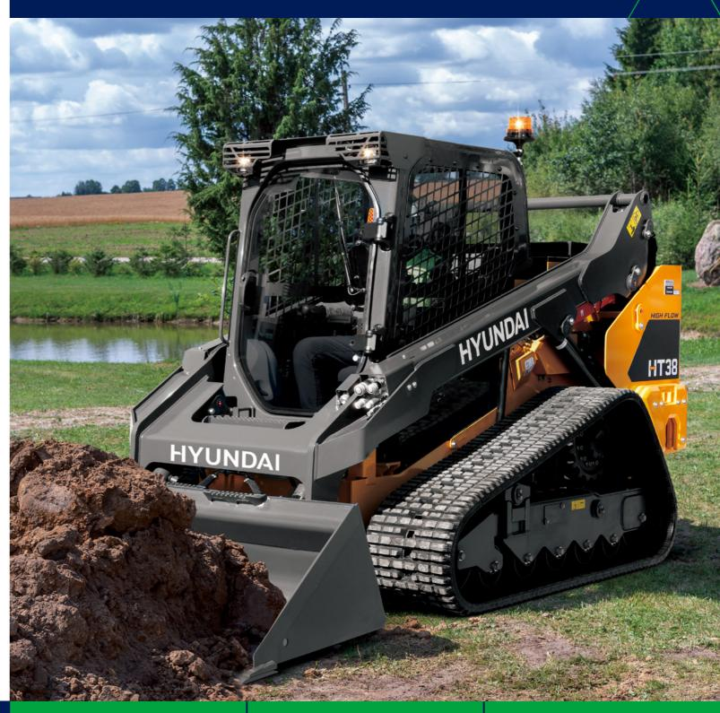
Engine Gross Power 115.3 HP (86 kW) / 2,400 rpm Rated operating capacity (35% of tipping load) 1,727 kg (3,806 lb) Operating Weight 5,799 kg (12,785 lb)
