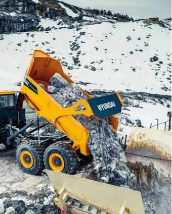
The optional heated body prevents frozen material sticking to it, enabling quicker and
