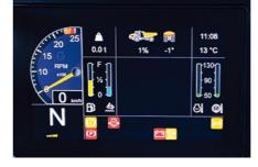
Multifunctional service and maintenance display makes it easy to check transmission oil level, plus hydraulic and electronic components.
