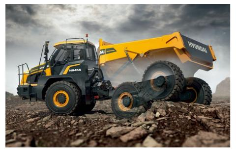
Front and rear differentials are limited slip while longitudinal differential can be manually locked.
