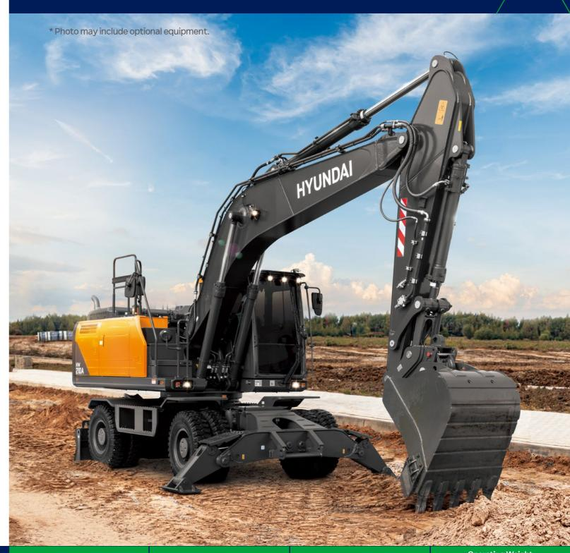
**Gross Power** 129 kW (173 hp) at 2,200 rpm
