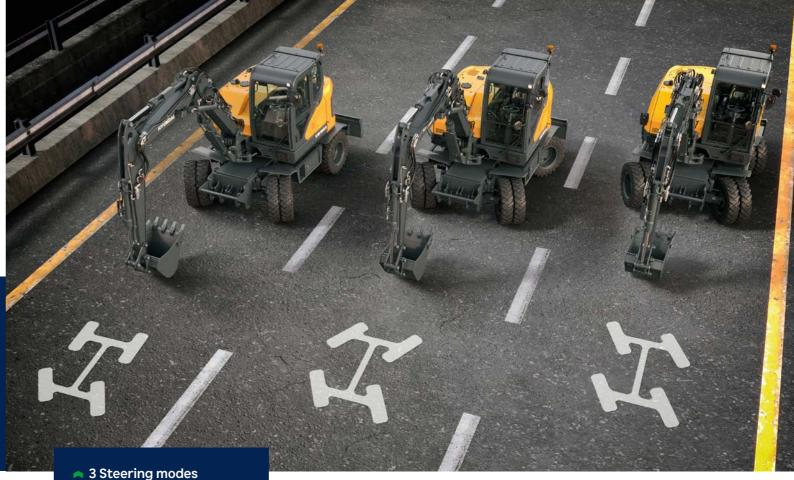
The optional 4-wheel steering increases the machine's manoeuvrability (including crab mode) and reduces its turning circle by 2m.
