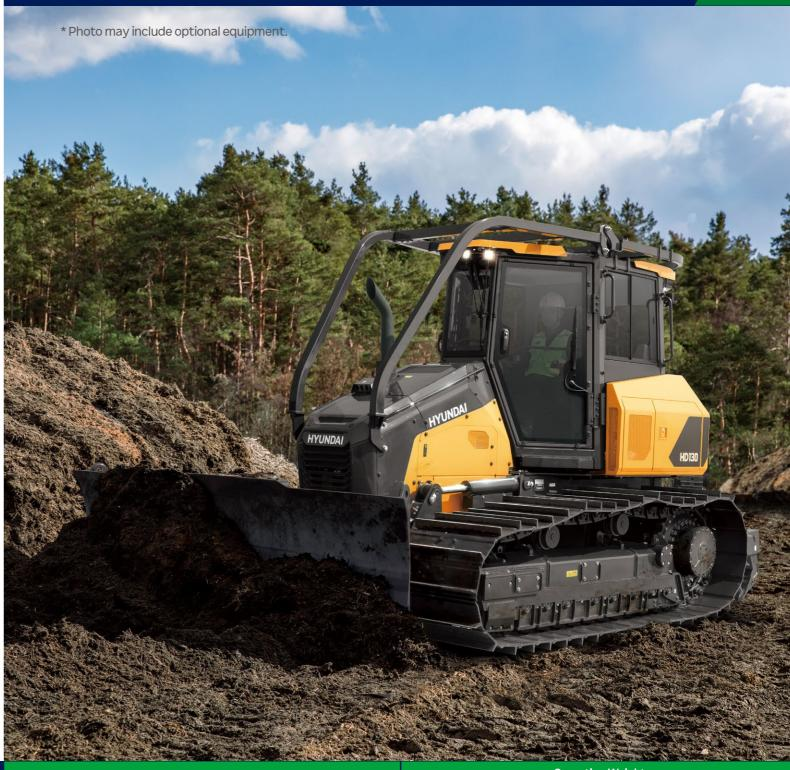
**Rated Power** 157 hp (117 kW) @ 2,200 rpm Operating Weight
