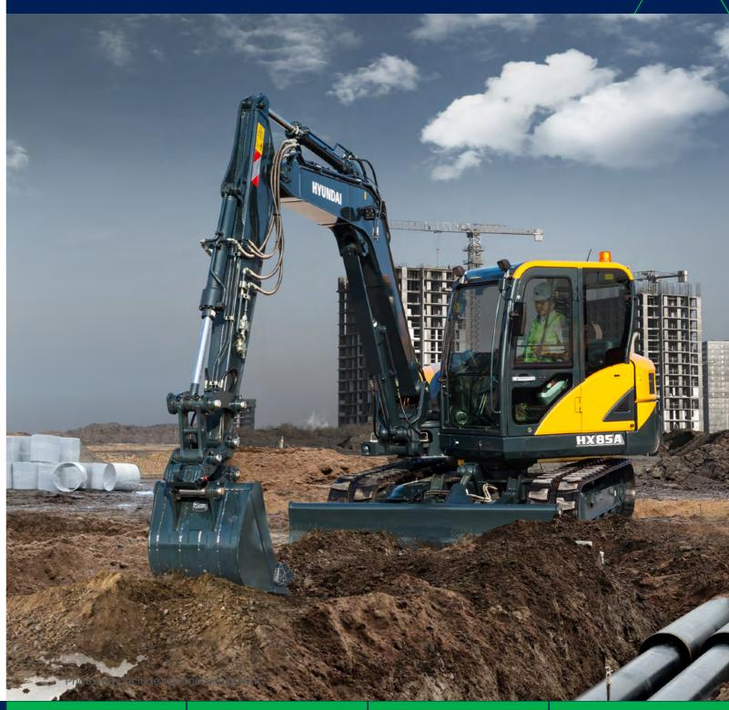
Gross Power (SAE J1,995) 66.9 HP (49.9 kW) at 2,400 rpm **Net Power (SAE J1,349)** 65.0 HP (48.5 kW) at 2,400 rpm Bucket Capacity 0.25m³ Operating Weight 8,950 kg / 19,730 lb
