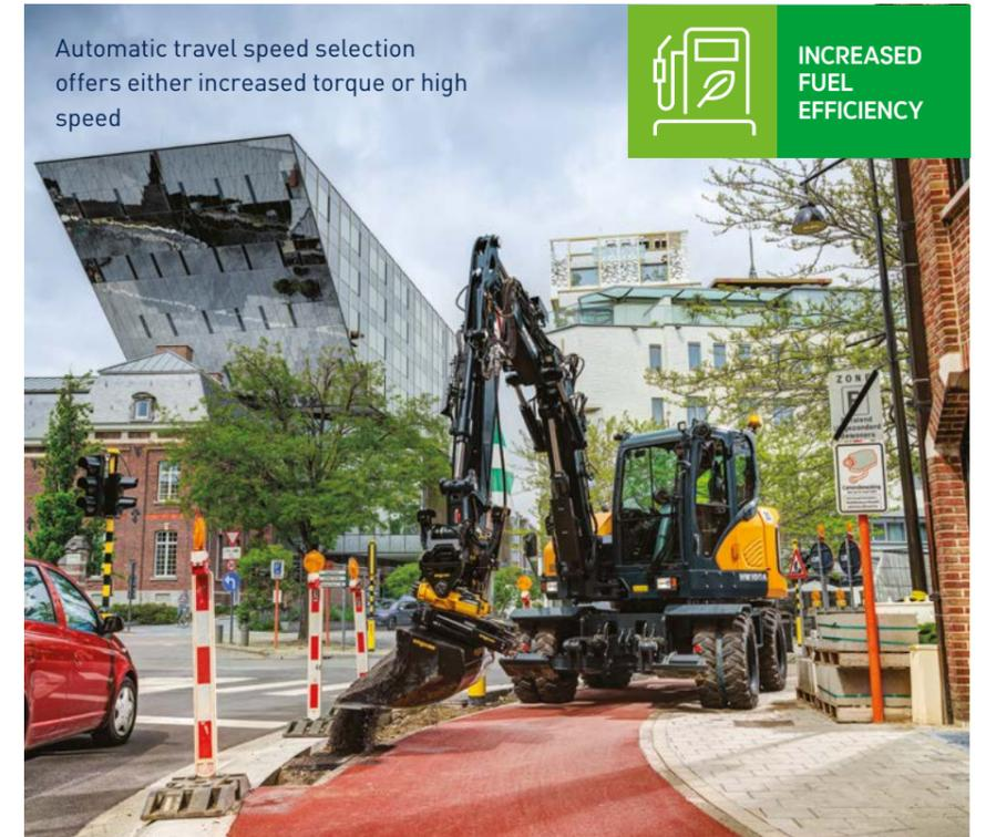
Automatic travel speed selection offers either increased torque or high speed
