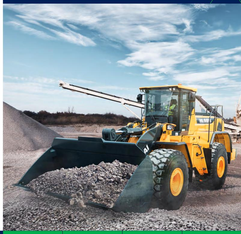
Gross Power (SAE J1,995) 335HP (250kW) at 2,100prm **Net Power** 330HP (246kW) at 2,100prm Bucket Capacity 5.6 m<sup>3</sup> Operating Weight 31,100 Kg (68,565lb)
