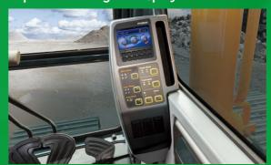
Instrument Panel is installed in front of RH console box. It is easy to check all critical systems with easy-to-read indicators.
