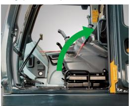
New joystick grips for precise control have been equipped with double switches.
