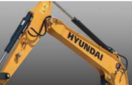
Standard breaker piping
