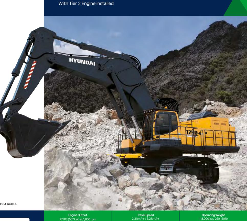
Engine Output 771 PS (567 kW) at 1,800 rpm **Travel Speed** 2.3 km/hr / 3.2 km/hr
