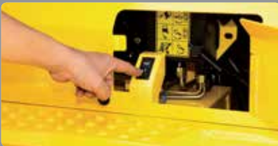
Cabin Air Fresh Filter The internal pressure is maintained to be slightly higher than that of outside to exclude dust and to reduce noise levels.
