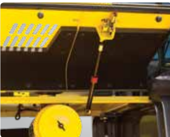
Automatic Self Locking Gas Spring Engine compartment hood is safely opened by a self locking gas spring.
