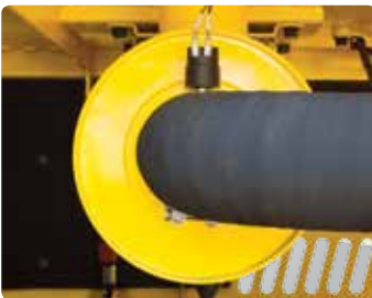
Electrically Monitored Air Filter Air cleaner sensor alerts the operator of a clogged air filter and allows replacement before damage.
