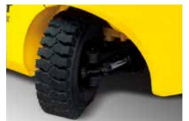
**Fully hydrostatic power steering**
